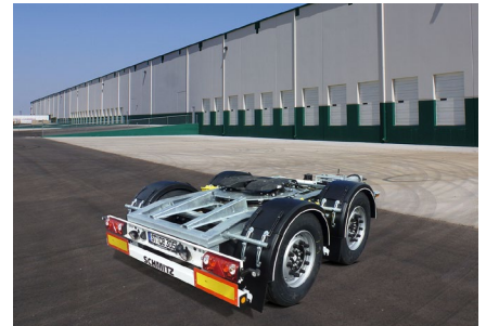
Dolly DO 18/L-2" The easy-to-use fifth wheel for the EcoDuo long-truck.
