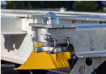
TWIST LOCKS with anti-twist lock on four pairs of container beams as standard.
