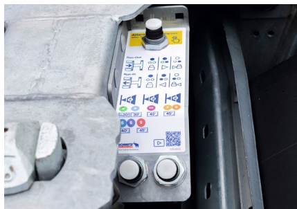
Control for the pneumatic rear extension , optionally with manual locking.
