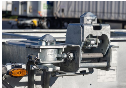
With 2 x 20' loads, the height-adjustable KLAPP LOCK takes over the locking of the front container.
