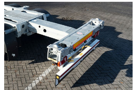
For more safety: New damped rear extension moves pneumatically to the selected locking position and brakes gently.
