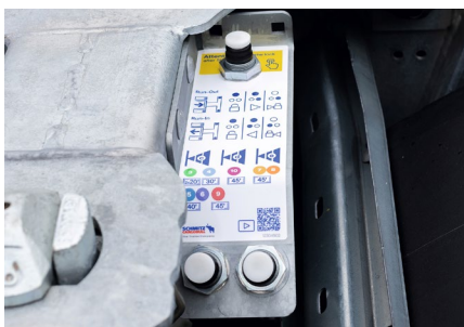
Control for the pneumatic rear extension with manual locking.
