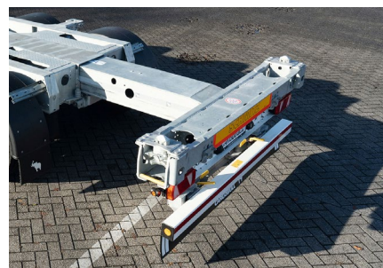
New: The rear extension moves pneumatically to the selected locking position and brakes gently.
