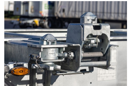
With 2 x 20' loads, the height-adjustable KLAPP LOCK takes over the locking of the front container.
