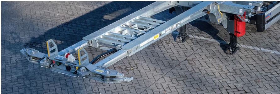
MULTI LOCK on the front beam with locking positions for tunnel containers with angled corners, straight corners and for containers without a tunnel, with positively guided plug-in locking.
