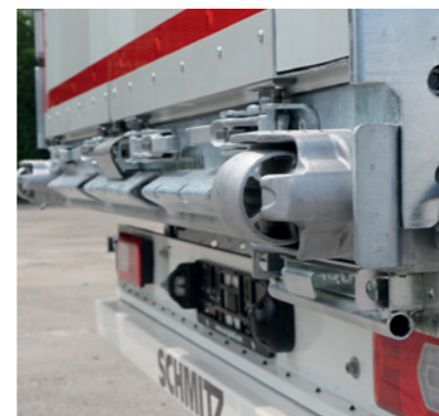
Ramp package Rear Package protects the rear portal and head frame from damage during loading. It consists of the reinforcement of the head frame in the chassis as well as Delta steel bumpers and compressible roller bumpers.
