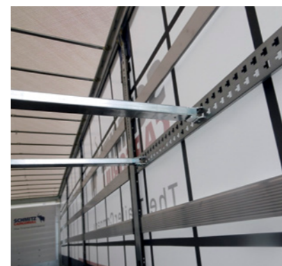
Load securing: A wide range of options, for example with a flexible load securing system.
