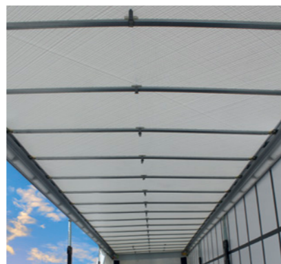
Schmitz Cargobull Safety Roof Integrated diagonal bracing increases body strength.
