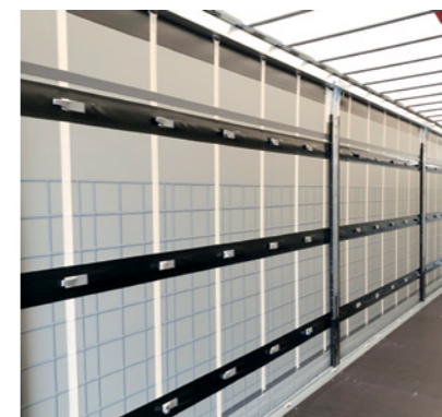
POWER CURTAIN*: Structure without top slats for shorter loading and unloading times and greater work safety.
