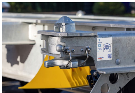
TWIST LOCKS with an anti-twist lock on four pairs of container beams as standard.
