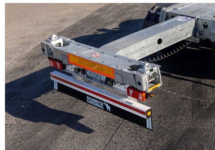
New: The damped rear extension moves pneumatically to the selected locking position and brakes gently.
