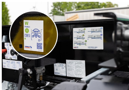
New operating concept with loading plan and clear function and warning notices on locks and extensions.
