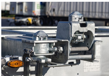
With 2 x 20' loads, the height-adjustable KLAPP LOCK takes over the securing of the front container.
