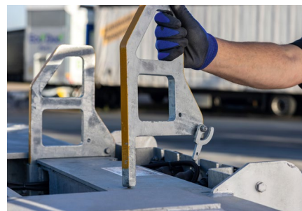
Easily replaceable container guides for containers on the front beam.
