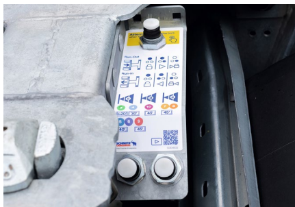
Control for the pneumatic rear extension with optional manual locking.
