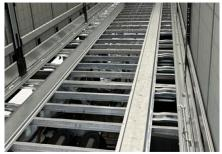
X-TOUGH chassis with high bending and torsional strength for 44 tonnes or more The S.CS X-TOUGH chassis impresses with its high bending and torsional strength. With its higher distributed load, optimised weight and a cross member spacing of max. 400mm, the MODULOS chassis offers greater strength reserves.
