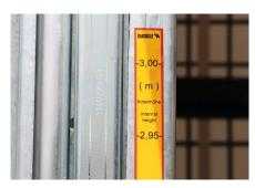
The height-adjustable **VARIOS body** ensures simpler and more flexible dispatch. The interior height is adjusted in two 50mm steps using plug-in strips.
