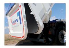
The surface-mounted **pendulum tailgate** with all-round seal is suitable for partial unloading and is optionally available with a sliding plate. The rear wall as an internal pendulum tailgate with a chute or a combination door extends the range.
