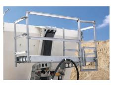
The **working platform** is used to operate the roller cover and is equipped with an anti-slip floor, a trough-shaped entry aid and a parking position for the hydraulic hose.
