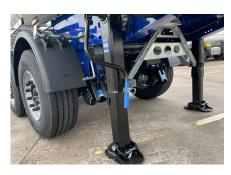
Secure standing with frequent changes of tractor: supporting winch or steel drop supports as full-load supports.
